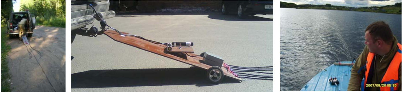
The towed facility of the RMT-M equipment with the fixed electric and magnetic sensors and preamplifier of electrical channels (at the left). Testing of boat-borne modification of the RMT-M equipment (at the right)
